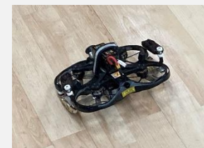
床下調査ドローン／DRONE VILLAGE
